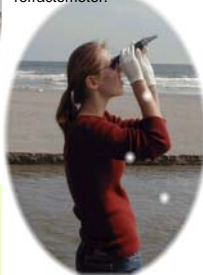
Nicole taking salinity reading with a refractometer.
