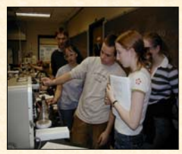
Andy Defobis, a student lab assistant, shows Marine Chemistry students how to use a salinometer to measure the salinity of their samples.
