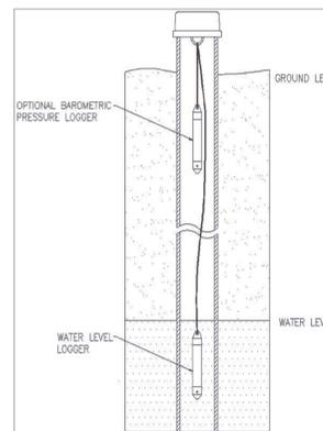
Figure 5: Stilling well design used in groundwater and lake wells. Graphic from Onset ([http://www.onsetcomp.com/files/manual\\_pdfs/12315-E-MAN-U20.pdf](http://www.onsetcomp.com/files/manual_pdfs/12315-E-MAN-U20.pdf))
